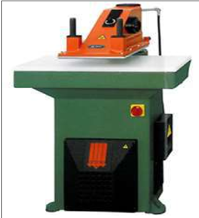
Fig. 5 Swing arm clicking press
