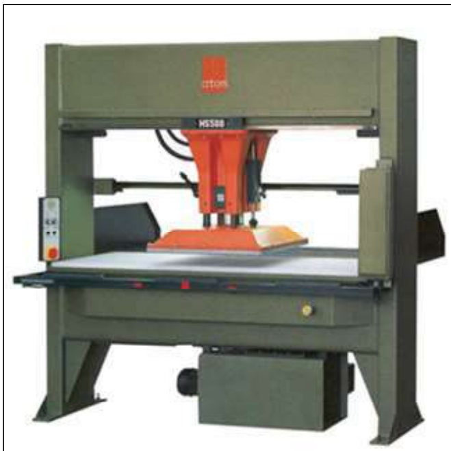
Fig. 6 Rotating head clicking press
