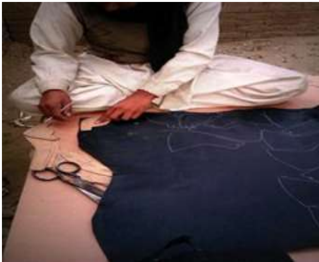
Fig.2 Upper clicking of components
