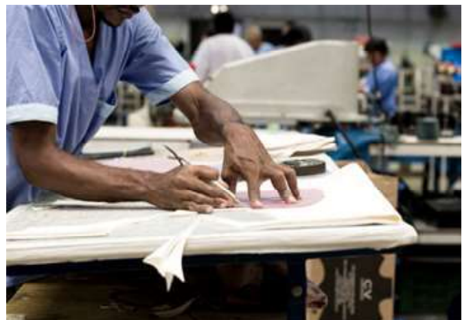
Fig. 4 Manual upper clicking with knife
