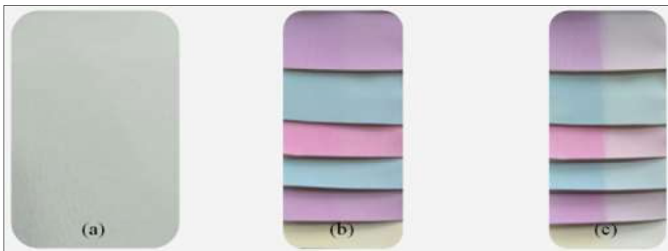
Figure 1 : (a) Polyurethane (b) Dyed polyurethane (c) Photochromic effect on polyurethane
