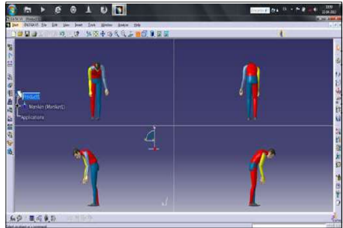
The backbone is tilted more than 66 degree causing harm to the human musculoskeletal system
