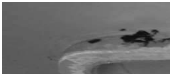
Fig. 4 GREY PICTURE OF SECTION OF A MOULD WHERE EVA MATERIAL IS HANGING AFTER REMOVAL OF PREPARED SHOE FROM MOULD
