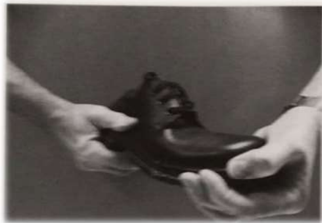
Method for manual assessment of torsional stiffness showing twist through length of the shoe.
