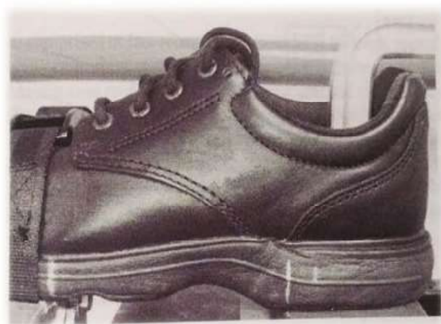
Torsional stiffness test rig setup showing front platform with central axis of rotation.
