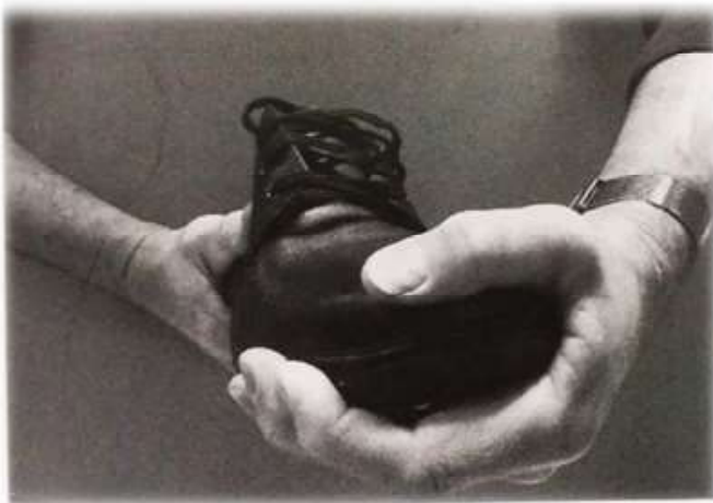
Method for manual assessment of torsional stiffness showing inversion of forefoot.
