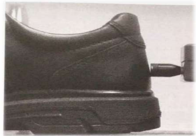
Alignment of soft-faced indenter at posterior aspect of heel counter.
