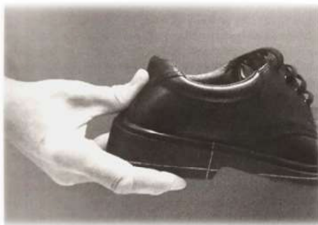
Method for manual assessment of heel counter stiffness
